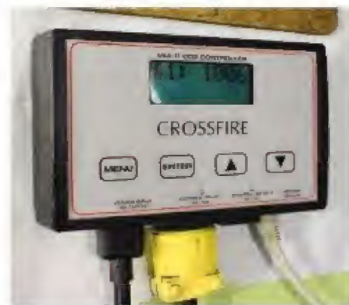
Digital meters must be used to monitor CO 2 levels (in PPM) in indoor gardens.
